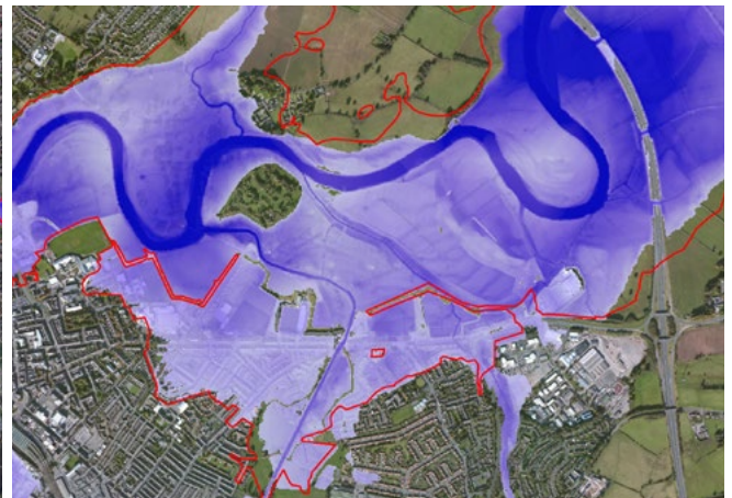
Carlisle – EA recorded flood event in red, monitoring layer output in blue.
